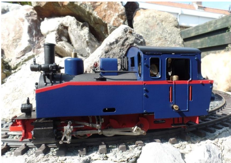
Roundhouse loco, rebuilt into an HF110C
