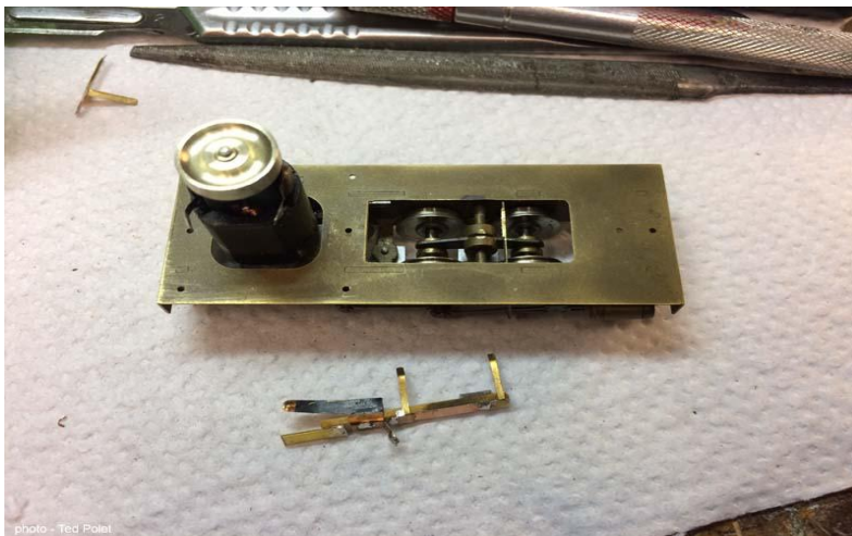
Frame of the steam locomotive, with pickups ready for installation:
